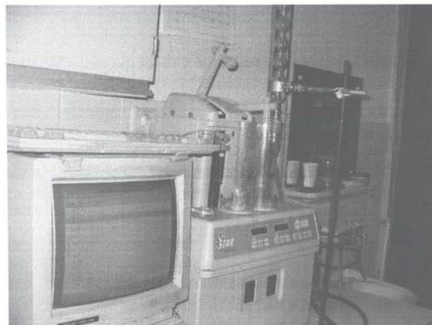
Fig. 1. The monomod microwave reactor STAR-2 for MW synthesis
